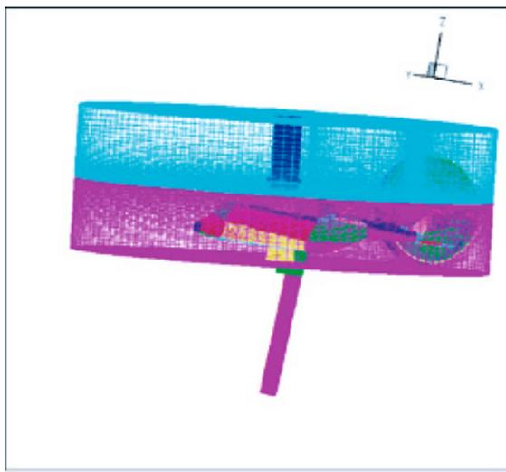
Fig. 1 The fuselage surface grid and the grids for the actuator disks.
