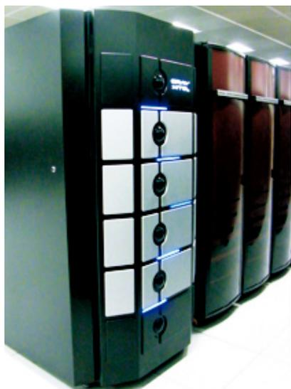
The Black Widow interconnection network has a point-to-point bandwidth of 16 Gb/s and a bi-section bandwidth of 254 Gb/s. The average ping-pong MPI latency is ~ 4.6  $\mu$ sec.
