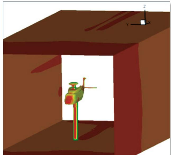
Fig. 4: Pressure contours on fuselage surface.
