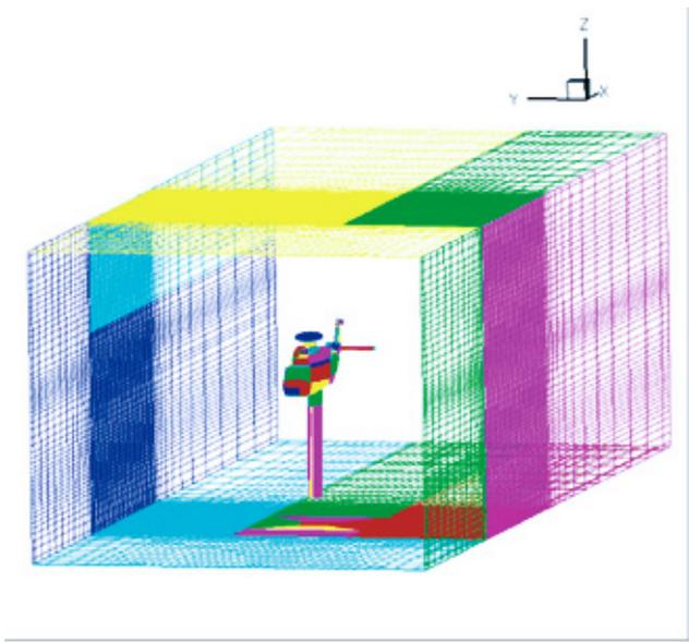
Fig. 3: The fuselage surface grid and the grids on the wind tunnel wall.
