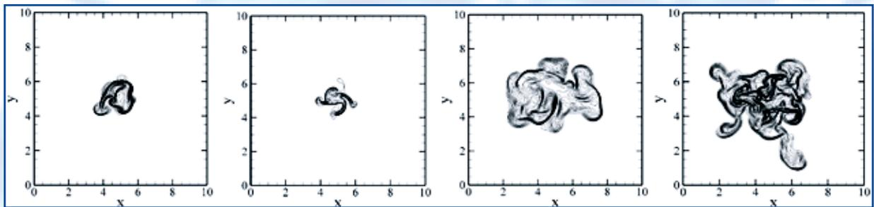
(a)  $z = 4$  plane  $\rho_l / \rho_g = 2.5$  (b)  $z = 4$  plane  $\rho_l / \rho_g = 5.0$  (c)  $z = 8$  plane  $\rho_l / \rho_g = 2.5$  (d)  $z = 8$  plane  $\rho_l / \rho_g = 5.0$
