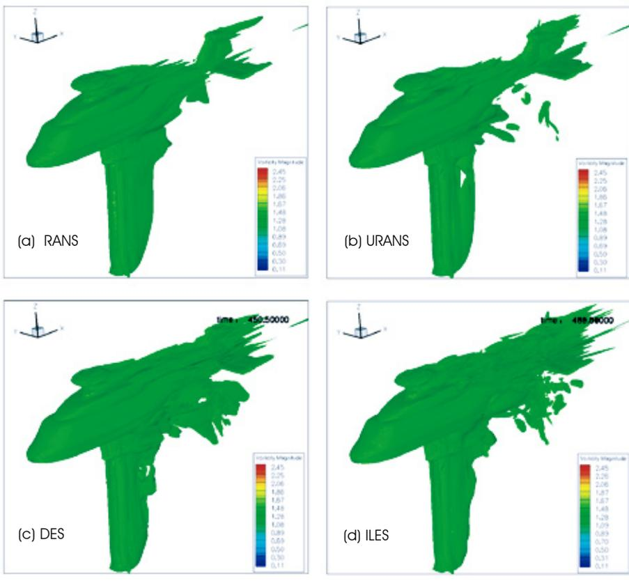
Figure 6. Vorticity iso-surfaces obtained using RANS, URANS, DES and ILES.
