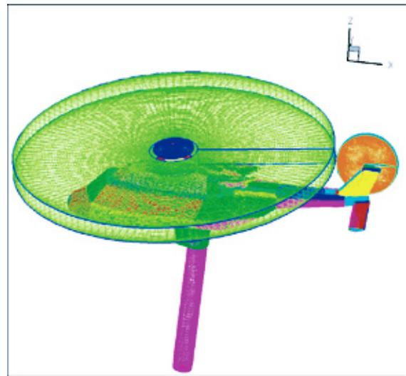
Fig. 2 Hole grids for Chimera approach.
