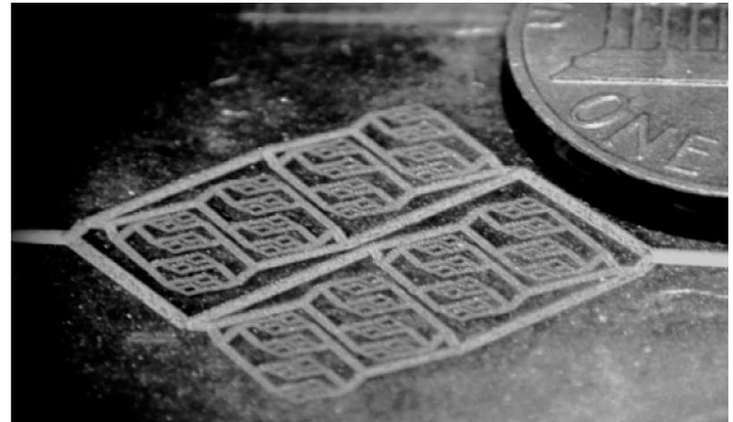
Eight generation multi-width and multi-depth microvasculature fabricated by Lim *et al.* (2003)
