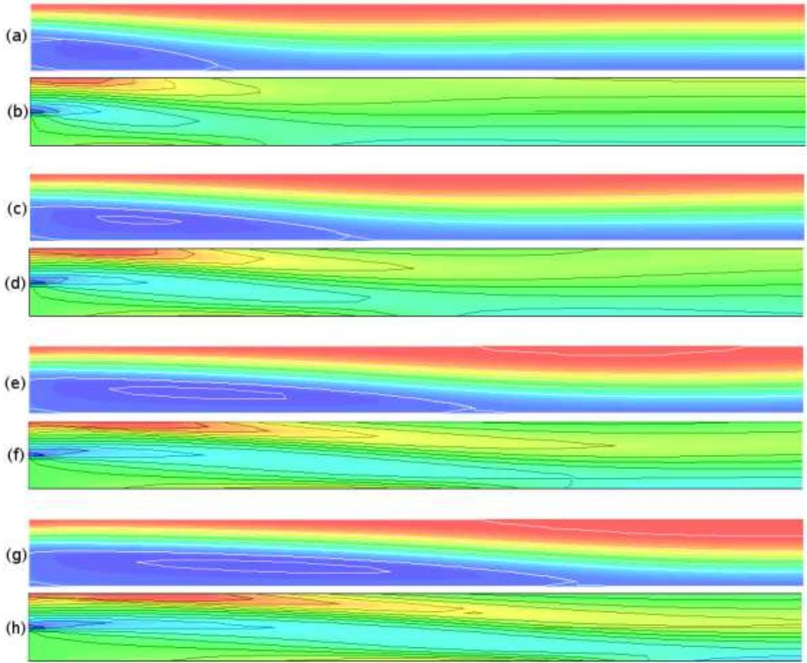
Figure 21: Streamfunction and Vorticity for the Backward-Facing Step.
